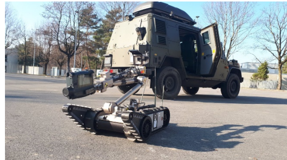
Figure 4 Reconnaissance robot equipped with a portable radiometry device
