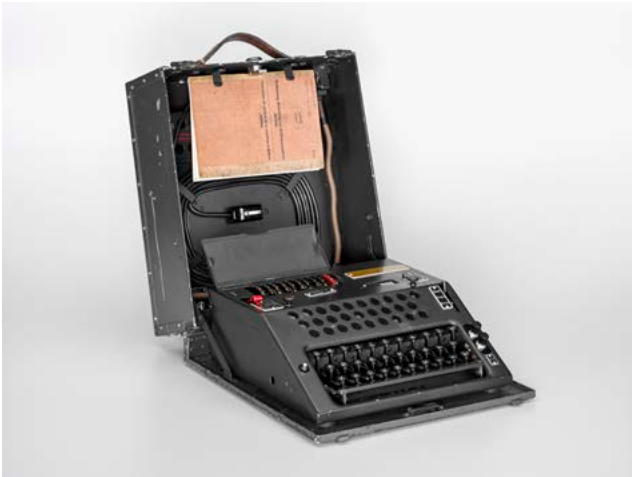
Illustration 1: NEMA rotor cipher machine of the Swiss Armed Forces and the Swiss Diplomatic Corps, used from 1947 to 1976. Training version. Complete with accessories. Manufacturer: Zellweger AG, Uster. (Source: Nationalmuseum SNM_DIG-48910_LM-176515.1-11)
